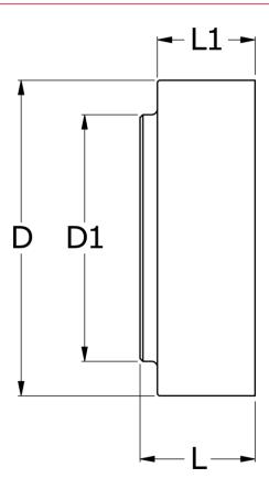
$\begin{array}{lll} D & = 400 \\ D1 & = 200 \\ L & = 160 \\ L1 & = 78 \\ Max bore & = 120 \\ Torque (N m) = 10300 \end{array}$
